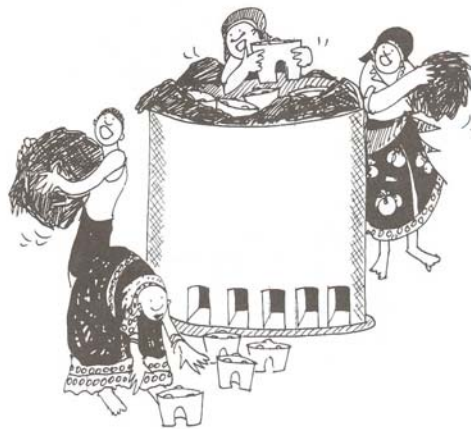
Figure 5.7 Unloading the kiln
