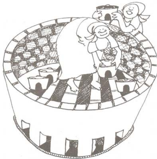
Figure 5.1 Loading the kiln
