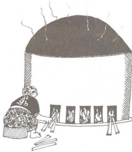
Figure 5.5 Feeding fuelwood into the fireboxes
